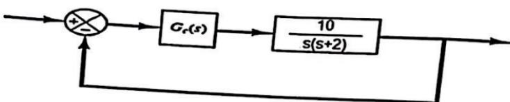
**b)** For the following control system, determine the value of the gain K such that the phase margin is 40°. [5 marks]
