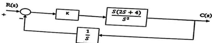
**Q3: a)** Obtain the state space model of the system shown in the following figure: [5 marks]
